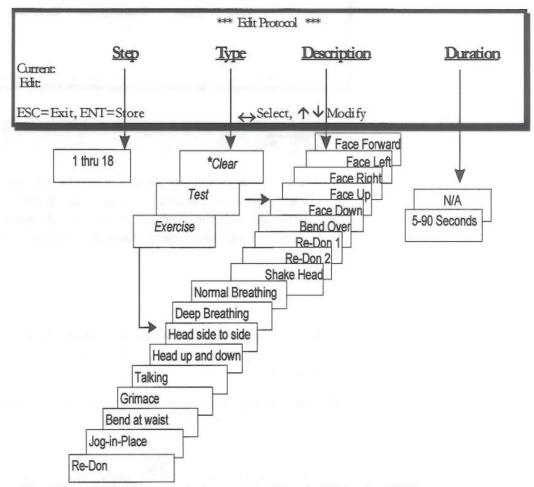
\*Select Clear ONLY at the end of a protocol. When the FitTester 3000 encounters a Clear, it does not advance to the next step. Instead it calculates results and shows a summary report. If all 18 steps are used, the additional step with Clear in the Type column is not necessary.
