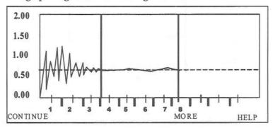
When the inhalation valve is not propped open or removed, the *FitTester 3000* is unable to get to the airspace touching the facepiece seal. The *FitTester 3000* is only looking at the seal of the inhalation valve, which can rapidly "flutter" with the sealing and breaking of the seal. The inhalation valve can easily be missed on some full-facepiece respirators that can be converted from SCBA or airline to Air Purifying Respiratory.
