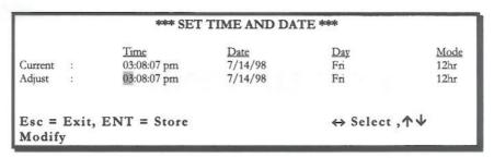
Use the ← or → keys to select the value on the "Adjust" line. Then use the ↑ and the ↓ keys to change the selected value.
