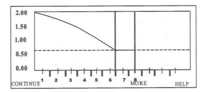
When the subject being tested continues to inhale after the squeeze bulb valve has been closed, it creates a negative pressure in the mask greater than needed for the test.
