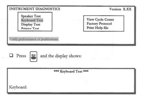
During this test, the keypad inputs are echoed to the display. When you press a key, the description of that key should show on the display.
