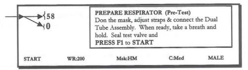
The two numbers in the upper left corner of the above-illustrated display indicate the challenge pressure and respirator mask pressure.
